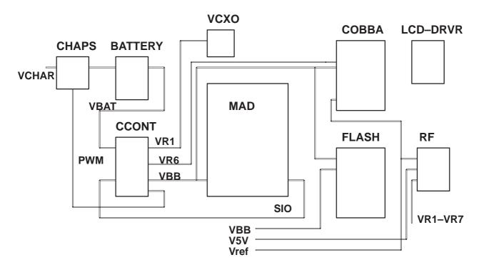
Battery voltage VBAT is connected to CCONT which regulates all the supply voltages VBB, VR1–VR7, VSIM and V5V. CCONT enables automatically VR1, VBB, VR6 and Vref in power–up.
