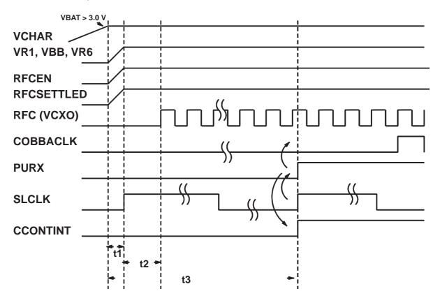
Before battery voltage voltage rises over 3.0 V CHAPS gives an initial charge (with limited current) to the battery. After battery voltage reaches that voltage limit the power up procedure is as described in the previous chapters.
