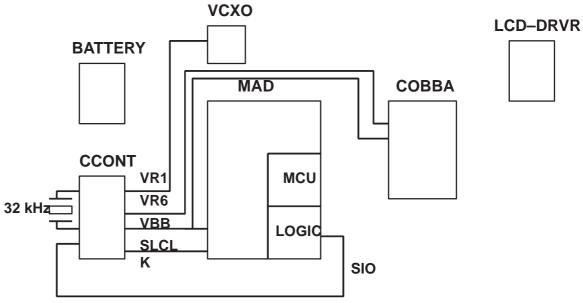
MAD must reset CCONT watchdog regularly. CCONT watchdog time can be set through SIO between 0 and 63 seconds at 1 second steps. After power–up the default value is 32 seconds. If watchdog elapses, CCONT will cut off all supply voltages.
