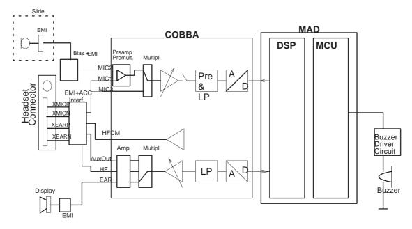
The baseband supports three microphone inputs and two earphone outputs. The inputs can be taken from an internal microphone, a headset microphone or from an external microphone signal source. The microphone signals from different sources are connected to separate inputs at the COBBA\_D asic. Inputs for the microphone signals are differential type.
