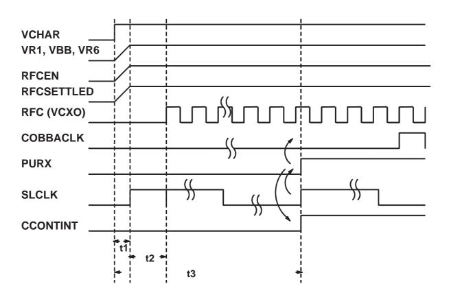
The power up procedure is similar to process described in the previous chapter with the exception that the rising edge of VCHAR triggers the power up in CCONT.
